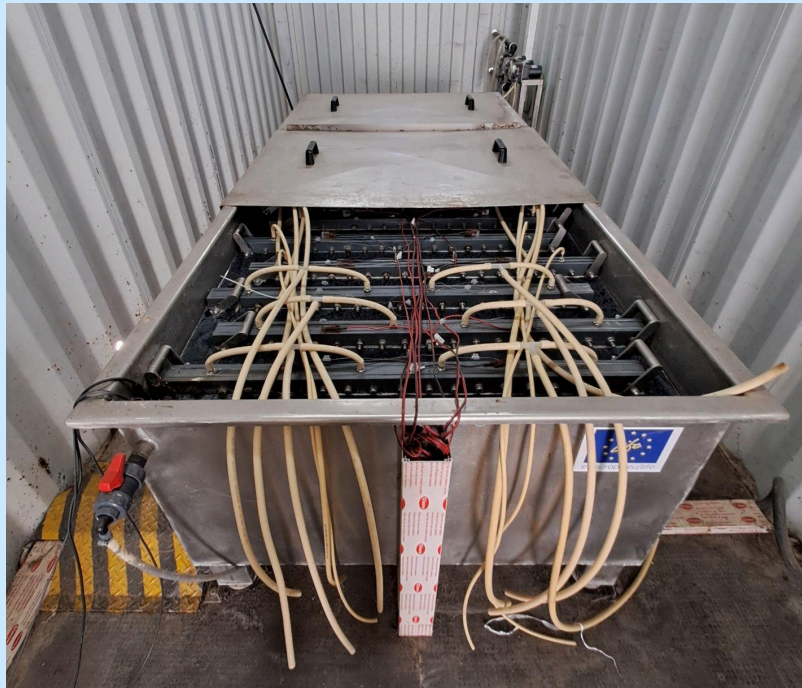
Figure 4. Detail of the cells arrangement of the BES unit
