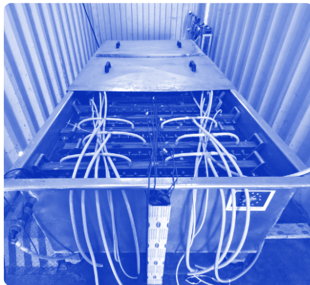
Image 4. Bio-electrochemical system that produces hydrogen for the biomethanation pilot plant within the LIFE NIMBUS site.
